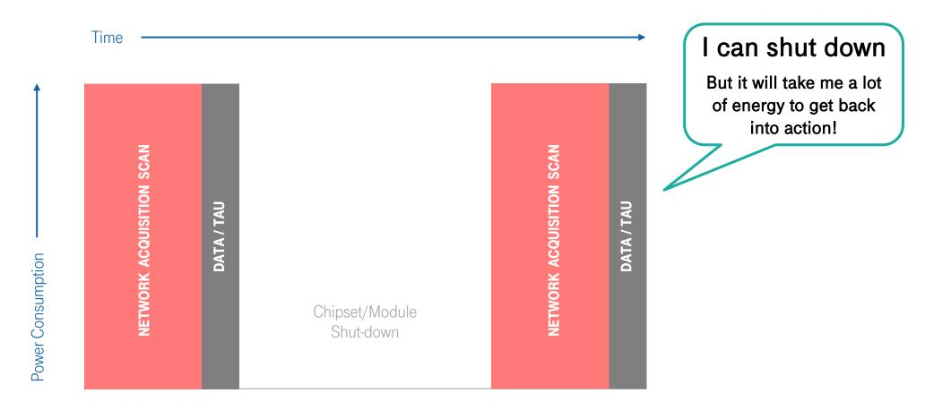
From observation, network acquisition scans of chipsets vary widely – taking from a few minutes to up to half an hour. Unless the period between messages is sufficiently long to compensate the power of such a network scan, use 3GPP<sup>TM</sup> power saving features instead.
