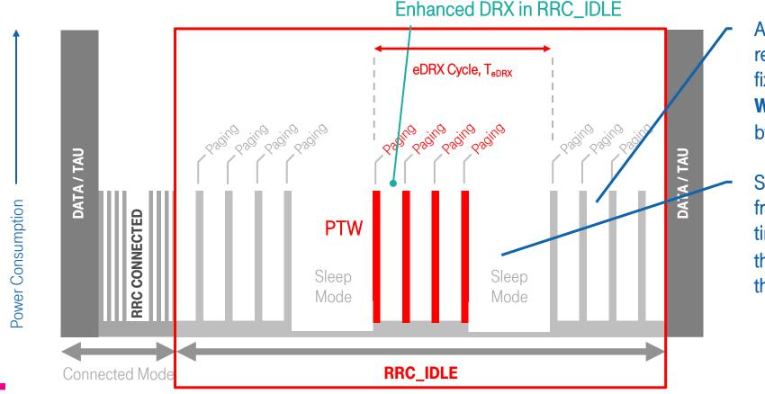
A DRX procedure (4-16 paging reception slots) is performed in fixed **Paging Transmission Windows (PTW)**, configurable by the IoT application
